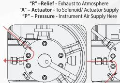
**Auto Mode** Pressurized supply air flows freely into "P" port and out "A" port to the Actuator/Solenoid.
