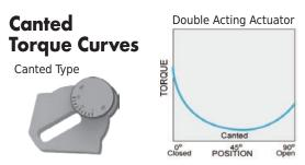
CHD series is equipped with a CANTED design yoke that produces a higher maximum torgue at the beginning of stroke (i.e. valve unseating/reseating at 0°) and less torque at the end of stroke (90°), therefore this series is optimal solution for high performance butterfly valves.
