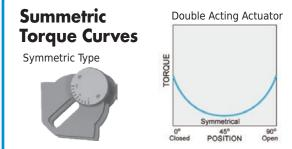
SHD series is equipped with a SYMMETRIC design voke that produces maximum torques at both ends of the stroke (0° and 90°) and minimal in the middle, therefore this series is the optimal solution for metal seated ball valves, plug valves and for modulating service.
