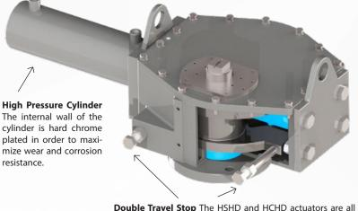
Double Travel Stop The HSHD and HCHD actuators are all provided with bi-directional travel stops to allow for open and closed position location adjustments of +/- 6 degrees.
