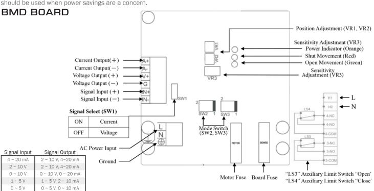
Note - When using current signal, external resistant is under 500  $\Omega_{\cdot}$
