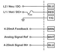
MAM Fail-Safe / Non Fail-Safe VAC/VDC Modulating
