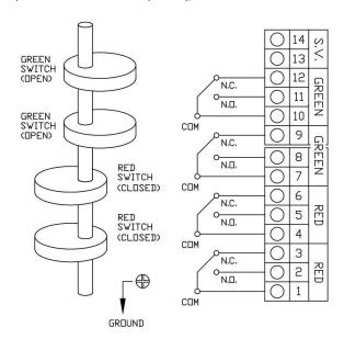
IS48: 2x Proximity sensors, 2 wires and 3 wires
