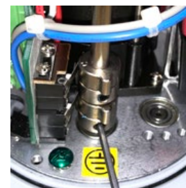
Fig 4 - CCW EOT Cam adjustment
