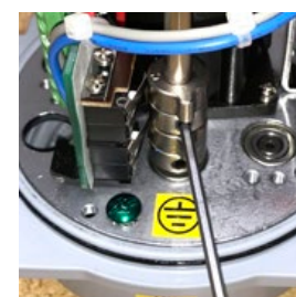
Fig 5 - CCW AUX Cam adjustment
