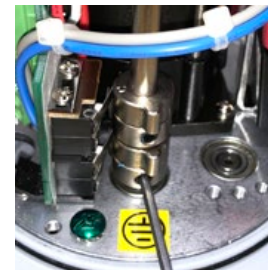
Fig 4 - CCW EOT Cam adjustment
