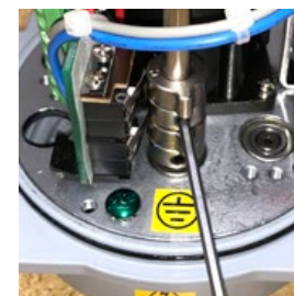
Fig 5 - CCW AUX Cam adjustment
