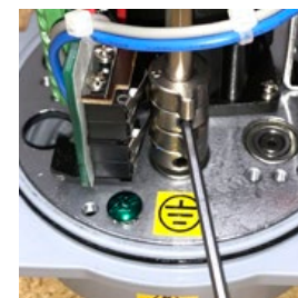
Fig 5 - CCW AUX Cam adjustment
