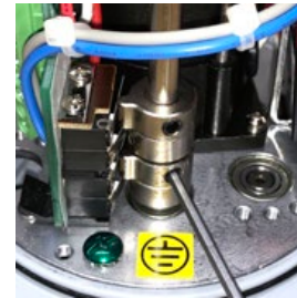
Fig 2 - CW EOT Cam adjustment
