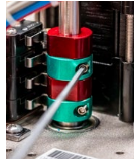
Fig 7 - CCW AUX Cam adjustment
