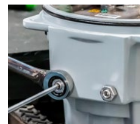
Fig 10 - Left side (CCW) mechanical stop
