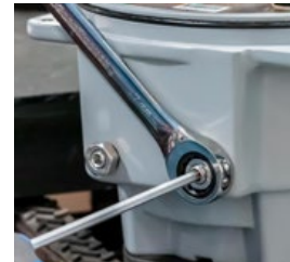
Fig 2 - Right side (CW) mechanical stop
