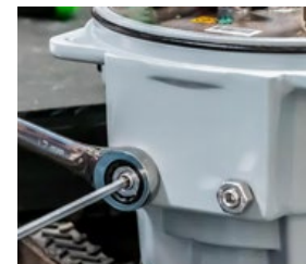
Fig 9 - Left side (CCW) mechanical stop
