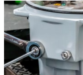
Fig 3 - Left side (CCW) mechanical stop
