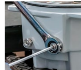
Fig 8 - Right side (CW) mechanical stop
