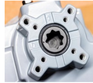
Fig 1 - Bottom view of actuator showing the "0" mark (Closed [CW] position), the "1" mark (Open [CCW] position), and the dimple reference. The actuator is shipped from the factory in its fully CLOSED position.
