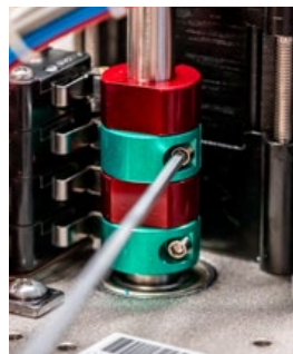
Fig 7 - CCW AUX Cam adjustment
