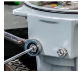
Fig 3 - Left side (CCW) mechanical stop
