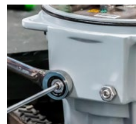
Fig 10 - Left side (CCW) mechanical stop
