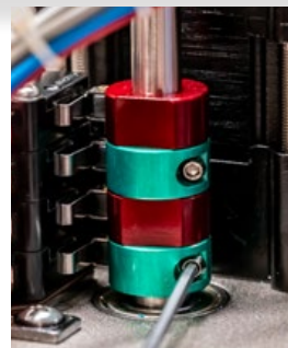
Fig 6 - CCW EOT Cam adjustment
