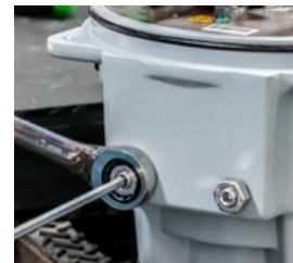
Fig 3 - Left side (CCW) mechanical stop
