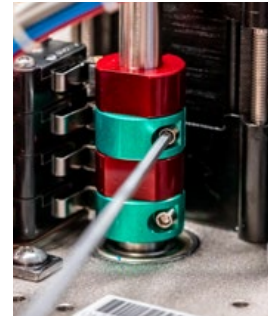
Fig 7 - CCW AUX Cam adjustment
