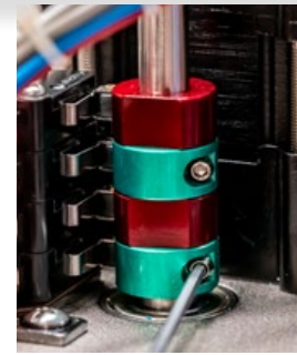
Fig 6 - CCW EOT Cam adjustment
