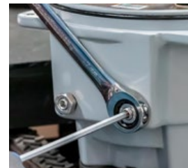
Fig 2 - Right side (CW) mechanical stop
