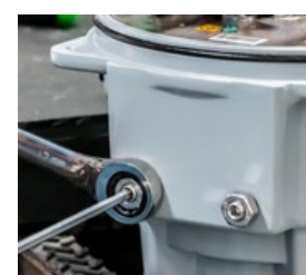
Fig 10 - Left side (CCW) mechanical stop
