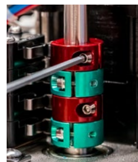
Fig 5 - CW AUX Cam adjustment
