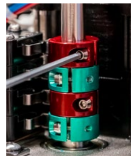
Fig 5 - CW AUX Cam adjustment
