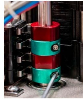
Fig 6 - CCW EOT Cam adjustment
