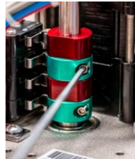
Fig 7 - CCW AUX Cam adjustment
