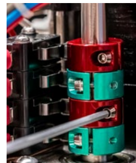
Fig 4 - CW EOT Cam adjustment
