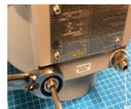
Fig 10 - Left side (CCW) mechanical stop
