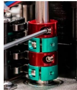
Fig 6 - CW AUX Cam adjustment
