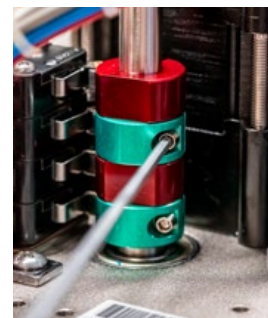
Fig 8 - CCW AUX Cam adjustment
