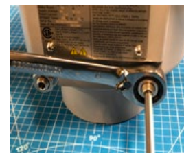
Fig 9 - Right side (CW) mechanical stop
