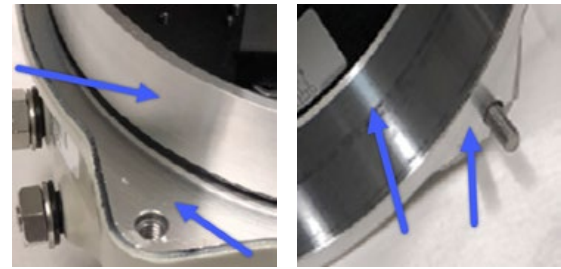
Fig 1 - Flame paths - Do NOT scratch, mar, dig or otherwise damage these surfaces!
