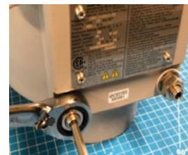
Fig 4 - Left side (CCW) mechanical stop
