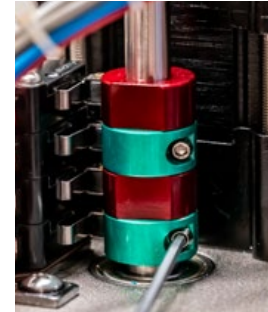
Fig 7 - CCW EOT Cam adjustment
