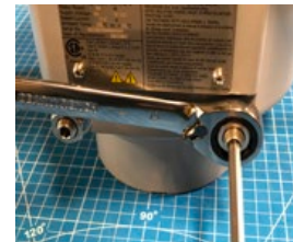
Fig 3 - Right side (CW) mechanical stop
