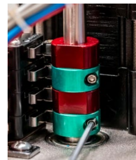
Fig 7 - CCW EOT Cam adjustment
