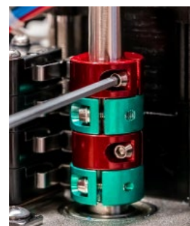
Fig 6 - CW AUX Cam adjustment
