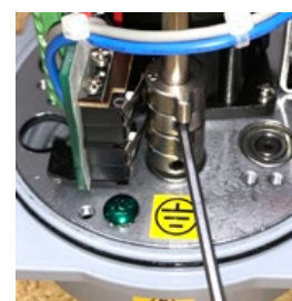
Fig 5 - CCW AUX Cam adjustment
