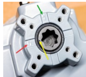
Fig 2 - Bottom view of actuator showing the "0" mark (Closed [CW] position - RED arrow), the "1" mark (Open [CCW] position - GREEN arrow), and the dimple reference (YELLOW arrow). The actuator is shipped from the factory in its fully CLOSED position.
