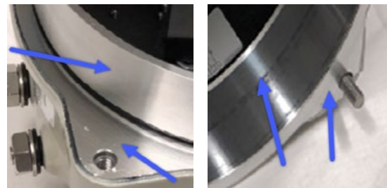
Fig 1 - Flame paths - Do NOT scratch, mar, dig or otherwise damage these surfaces!
