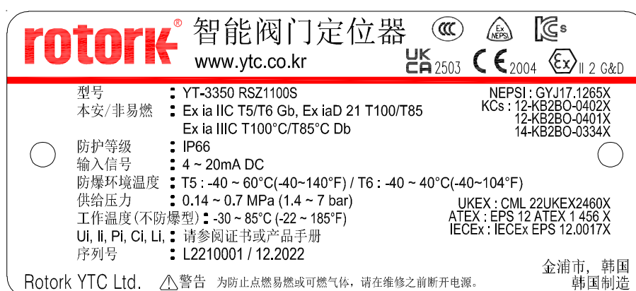
Fig. L-16: YT-3350 Intrinsic safety type (CCC)
